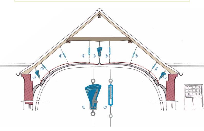
The various low tension force regulators were specially developed for load regulation of components in a certain expansion range (up to 500 N), e.g. for use on suspensions of wire plaster vaults and ceilings.
